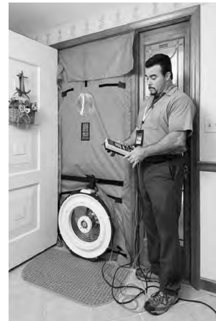
Blower door technology measures home air leakage.
