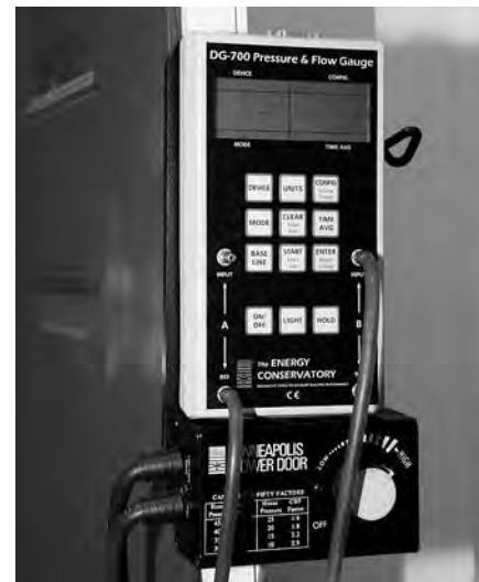
Blower door test readings indicate the tightness of a homes envelope and the process reveals drafts and leaks to be fixed.
